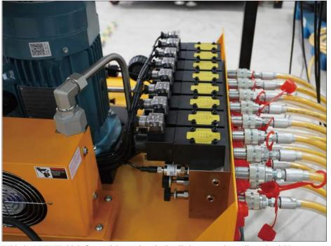
With the ULTPER high-flow quick couplers, hydraulic hoses can be easily and quickly connected to the PLC-controlled synchronous jacking hydraulic system.
