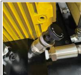
Loosen the lock nut on the relief valve and slowly turn the relief regulator clockwise so that port A reaches the target pressure.
