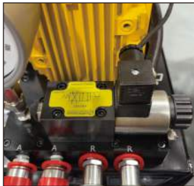
Through the solenoid valve control button on the handle, the system oil flow direction is accurately controlled.
