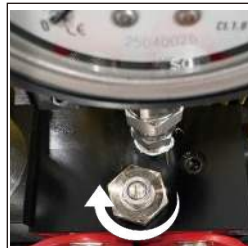
The return pressure is regulated by the R-port pressure limiting valve
