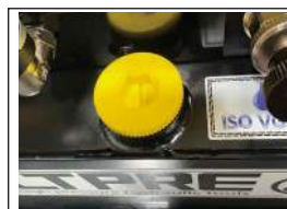
If the oil level is lower than two - thirds, remove the plug and then carry out the oil - filling operation.
