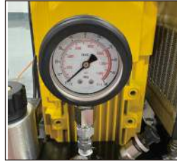
Under no-load condition of the system, confirm that the initial reading of the pressure gauge is zero.
