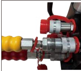
The oil pipe is fully pushed into the outlet by axial alignment
