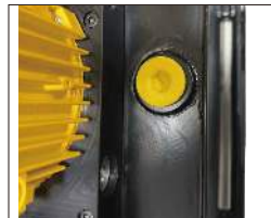
If the oil level is lower than 2 / 3, rotate the oil outlet.
