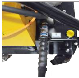
After pushing the oil pipe, push the outer lock ring forward and rotate it clockwise to lock.
