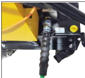
The outer lock ring is pushed back, and the oil pipe is fully pushed into the outlet by axial alignment.
