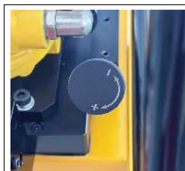
Loosen the lock nut on the relief valve and slowly turn the relief regulator clockwise so that port A reaches the target pressure.
