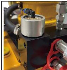
The pneumatic control valve on the handle is used to control the flow direction of the system oil accurately.
