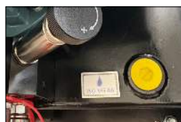
If the oil level is lower than 2/3, please rotate and remove the plug of this out-let, and then carry out the refueling operation.
