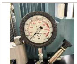
Under no-load condition of the system, confirm that the initial reading of the pressure gauge is zero.
