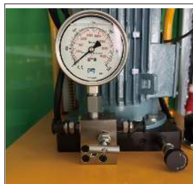
When depressurizing, hold the solenoid unloading valve on the handle and reduce the system pressure to the pressure indicator number 0.
