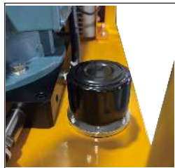
If the oil level is lower than 2/3, please rotate out the plug of this outlet and carry out the refueling operation.
