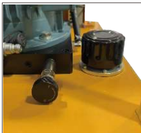
Loosen the locking nut to adjust the overflow pressure.
