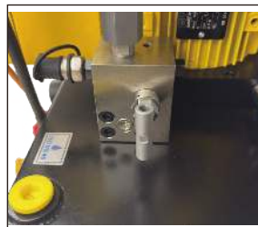
Slowly open the unloading valve when depressurizing, and reduce the system pressure to the pressure indicator number 0.
