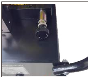
Loosen the locking nut to adjust the overflow pressure.
