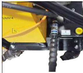
After pushing the oil pipe, push the outer lock ring forward and rotate it clockwise to lock.
