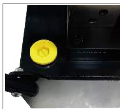
If the oil level is lower than 2/3 of the upper oil gauge scale line, the outlet plug should be removed and the hydraulic oil replenishment operation should be performed.
