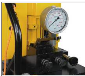
The hand-controlled directional valve has two working oil ports A and B. Push the valve stem to the corresponding gear to realize the switching of oil direction.
